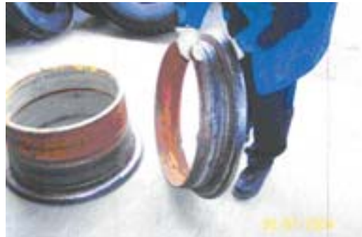
Figure 3: Assembly of wheel components. Rim base and flange on the ground; second flange being fitted; bead seat band between feet of fitter.
