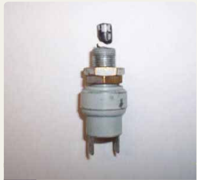
Switch with broken plunger.
