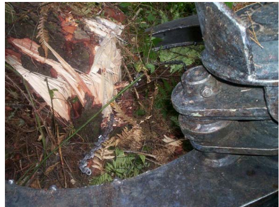
Felling head showing broken chain
