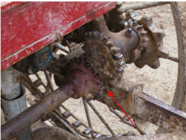
Photo 2: in-running nip point on ridger
