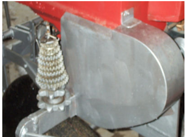
Photo 3: Possible guarding solution (Visible gear wheels are not in use)
