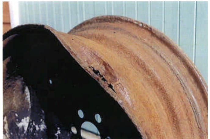
Photo of the wheel rim showing rust holes and folding in of rim edge.
