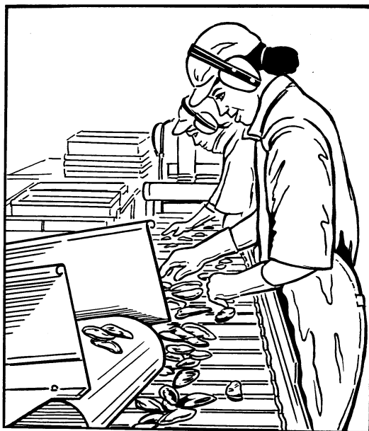
Workstation designed so that work can be performed close to the body.
