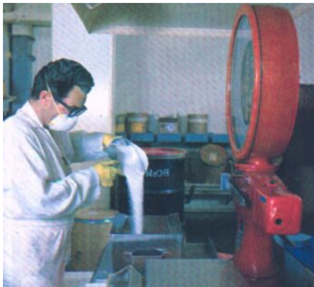
Worker wears face mask to avoid breathing dust while weighing solid caustic soda
